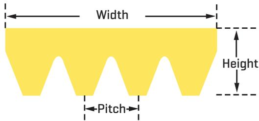
$$\text{Pitch} = \text{Belt width} / \text{Number of ribs}$$
