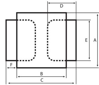
The principal dimensions of a EuroGrip® sleeve are the outside diameter, the sleeve length and the total coupling length. Gates EuroGrip® couplings are made in sizes 19, 28, 42, 48 and 60.
